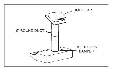
Straight up through the roof using 5" round duct (for single story installations only). Use a Model P85 5" round damper (sold separately).
