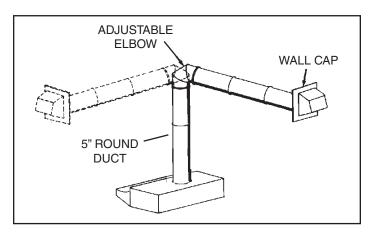
Ducting between the ceiling joists (for multi-story installations) or through the soffit space above the cabinets (where the soffit connects to an outside wall).
