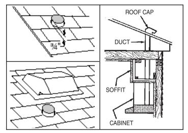
**Roof Cap Discharge:** Cut a hole in roof slightly larger than duct size being used. Run ductwork down to hood location. Leave 3/4" of duct projecting above roof surface on high side. Trim duct parallel to roof pitch and seal all around duct with roof cement.
