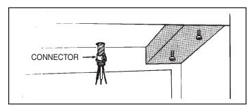
Run electric wiring through hole drilled in wall or cabinet. Split wiring for 6" and install proper connector for type of wire used.
