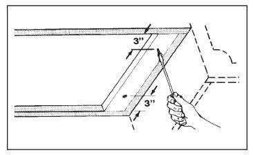
(For installation on recessed bottom cabinets only) Attach a wood filler strip at each side of recessed area under cabinet. Use two 1" x 2" strips cut to length. If recess is deeper than 1" use thicker strips. Attach strips with 1-1/4" wood screws, 3" from each end of strip.
