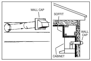
**Wall Cap Discharge:** Use saber saw or keyhole saw to cut hole slightly larger than duct size used so that duct will line up easily with damper/duct conector on hood. Install casing strips if cap will be installed on siding. Attach required amount of duct to wall cap and run duct back to hood. Fasten cap to wall and caulk well.
