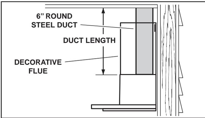
8. Measure and install steel ductwork to hood duct connector. Use duct tape to make all joints secure and air tight.
